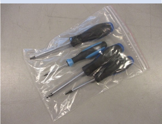
PAL3 Torx Tool Kit • Torx Screwdriver 8 mm (1 piece) • Torx Screwdriver 10 mm (1 piece) • Torx Screwdriver 20 mm (1 piece) • Torx Screwdriver 25 mm (1 piece)
