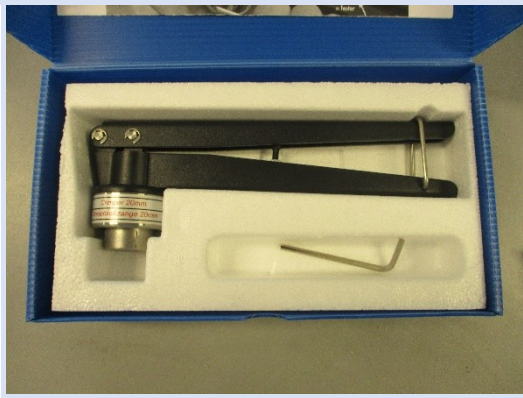
Crimper for 20 mL Headspace Vials
